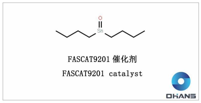
Product application: used as a catalyst for esterification and polymerization. Production methods and others: There are two main industrial methods:
